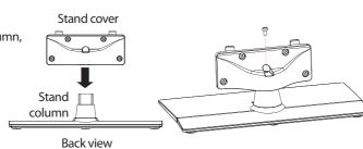
**4** Secure the stand cover to the TV using four M5 × 12 mm screws (provided).
